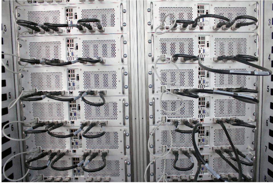
Fig. 4. Close-up view of the Janus II machine installed at BIFI (Zaragoza). The installation has 16 Janus II boxes (12 are visible in the picture). The cables supporting the data-links in the z direction are mounted in loop-back mode for test purposes.
