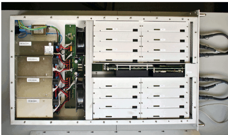
Fig. 3. Picture of a Janus II box; there are 16 SP modules (plugged vertically on the printed circuit), while the CP module is at the center of the structure; on the left one sees the cooling fans and the power supplies.
