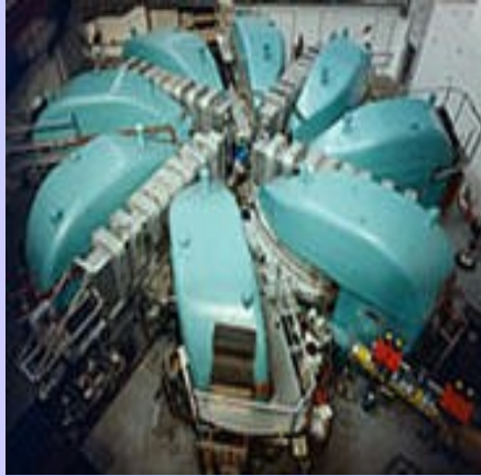
2.0mA, 590 MeV proton cyclotron
