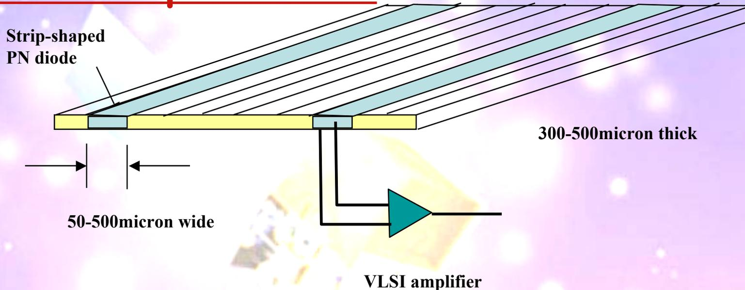
**Stable particle tracker that allows micron-level tracking of gamma-rays**
