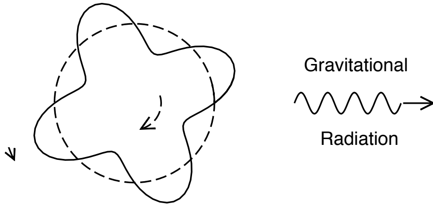
Figure 1.1. Oscillation mode (solid line) rotates in the direction opposite to the star rotation (dashed line). If the oscillation is dragged to move in the direction of star rotation, gravitational wave emission lead to instability.
